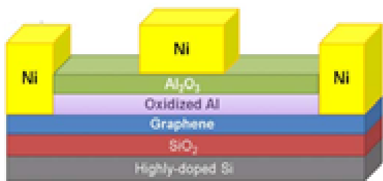
Figure 12. Structure of top gated graphene field-effect transistor [16] is used in our simulations.
