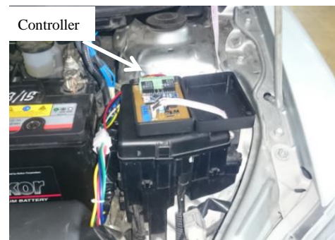
Figure 23. Control circuit is located under the bonnet
