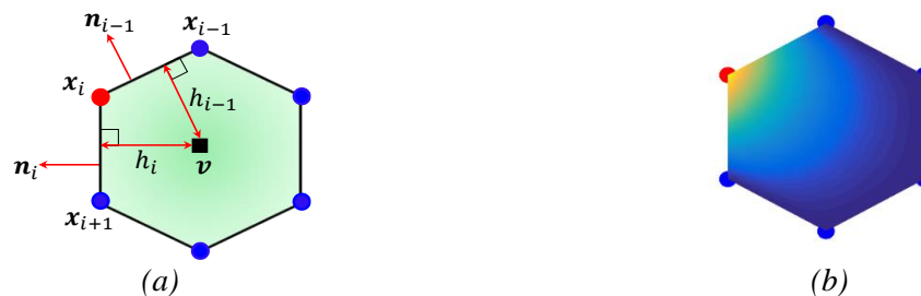
Figure 2. Wachspress shape functions for polygonal element: (a) Definition of Wachspress coordinates; (b) Wachspress shape function
