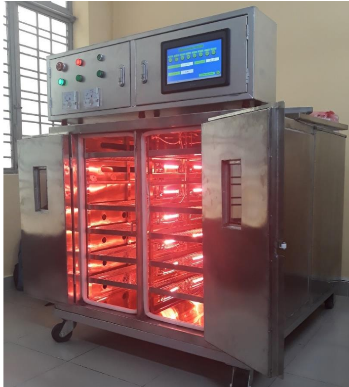
Figure 5. The manufactured smart infrared drying system with the capacity of 12 kg of materials per batch
