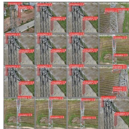
(b) Detected insulators by Yolov5x
