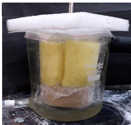
Fig. 3. Image of the jacketed vessel with PU-Salt PCM/PU-Gel PCM as an insulation layer
