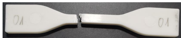
Fig.7. Samples after tensile testing
