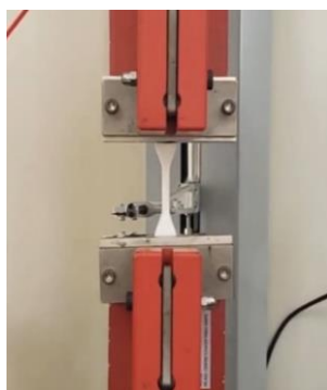
Fig. 6. Tensile strength testing process
