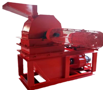
Fig.5. Construction of the Hammer Mill.
