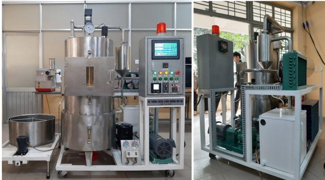
Figure 2. The manufactured vacuum frying system, DVF-03, with the initially designed requirement
