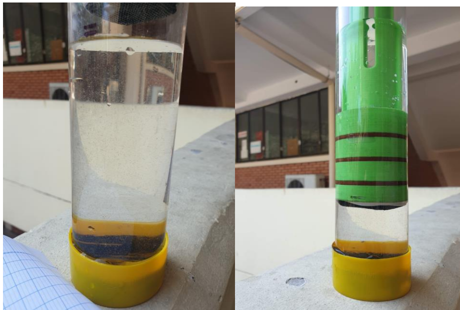
Figure 9. Water before and after filtration by portable device
