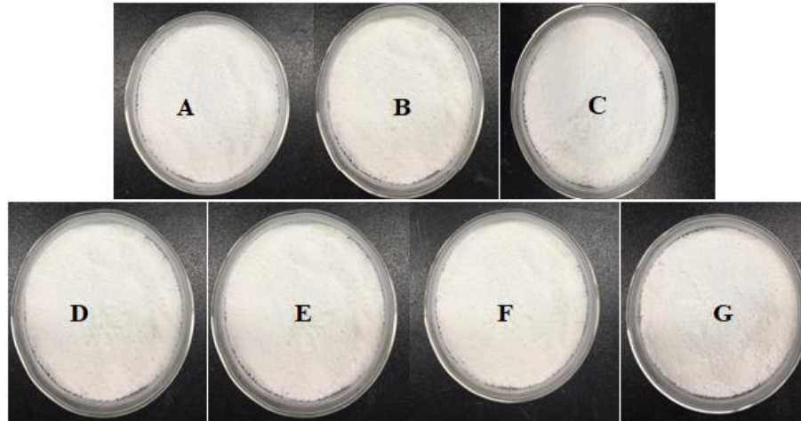
Fig.4. SOC70 sample at A (room temperature) and after 1 h at B (40 °C), C (50 °C), D (60 °C), E (70 °C), F (80 °C), G (90 °C)
