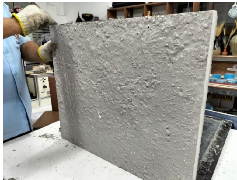
Figure 7. Forming of geopolymer insulator by synthesis of fly ash, waste powder coating and PU foam
