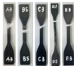
Figure 6. Tensile test samples of five materials after experiments
