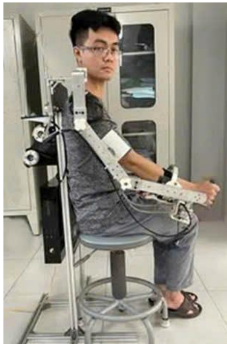
Figure 8. Prototype of the wrist exoskeleton
