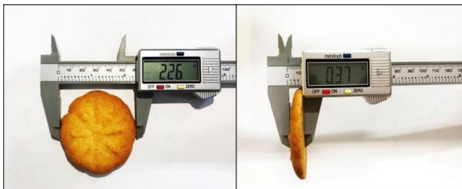
Figure 1. Demonstration of diameter measuring (left) and thickness measuring (right)
