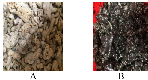
Fig. 3. Coral media before and after use for treatment (A: Initial coral, B: Coral in the tanks)
