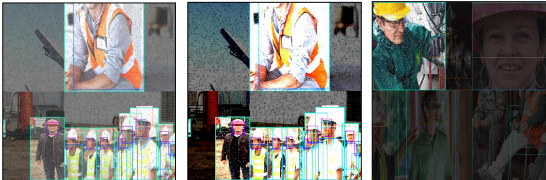
Figure 3. Image noise, mosaic, bright and dim light are applied during data augmentation process.
