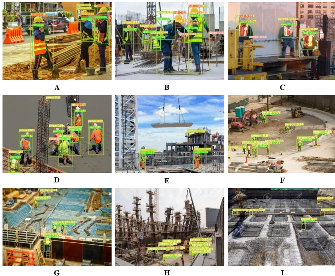
Figure 7. Testing result of YOLOv8l in different background and distances. (A, B, C) Objects in close distance, (D, E, F) Objects in medium distance, (G) Objects in far distance, (H, I) Object in far distance with complex background.
