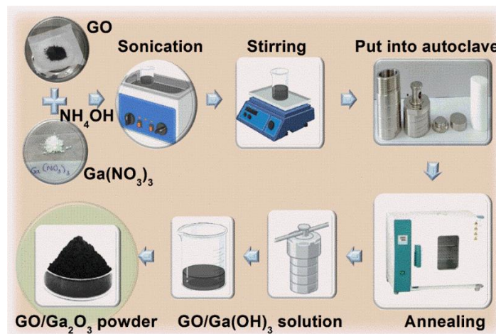
Figure 2. Schematic of preparing GO/ \text{Ga}_2\text{O}_3 composite using hydrothermal method.
