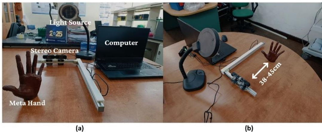
Figure 5. The experimental configuration for evaluating the accuracy of hand feature point reconstruction: (a) The experiments included a printed meta hand, a stereo camera, a light source, and a computer; (b) the printed meta hand was put 38 – 45 cm away from the left camera.
