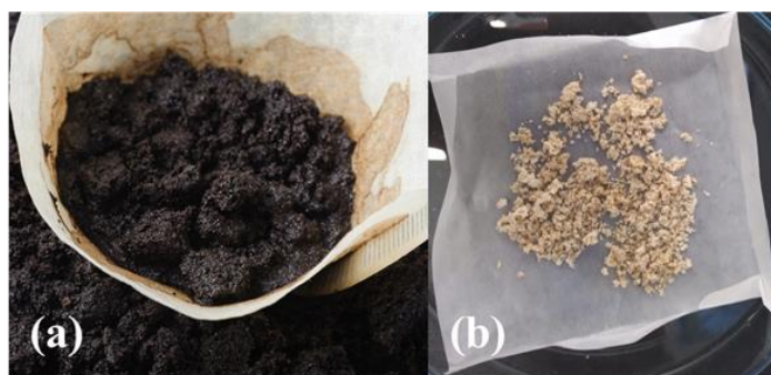
Figure 2. (a) The coffee grounds and (b) the extracted cellulose fibers.
