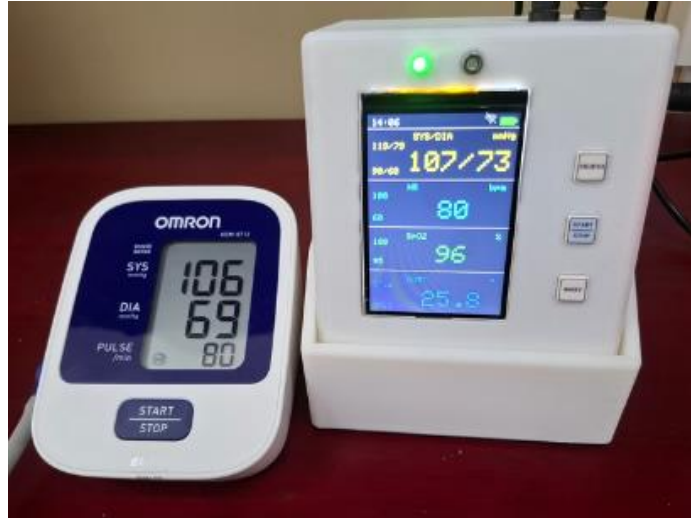
Figure 5. Compare blood pressure measurement results with OMRON machine
