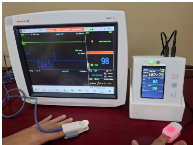
Figure 7. Heart rate and SpO 2 results compared with OMNI II
