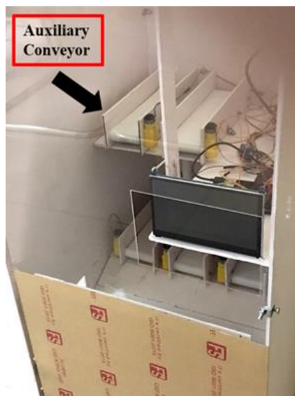
Figure 10. Auxiliary loading conveyors.
