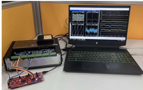
Figure 3. HIL experiment setup.
