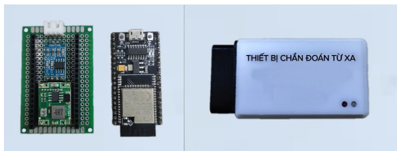
Figure 4. CAN communication module via OBD-II port
