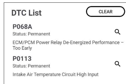
Figure 10. Results after clearing DTC on Ford Focus 2019
