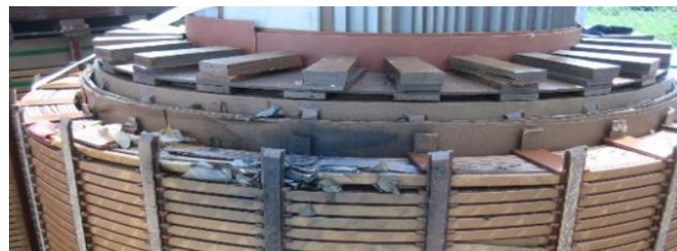
Figure 9. Short circuit inside the winding.
