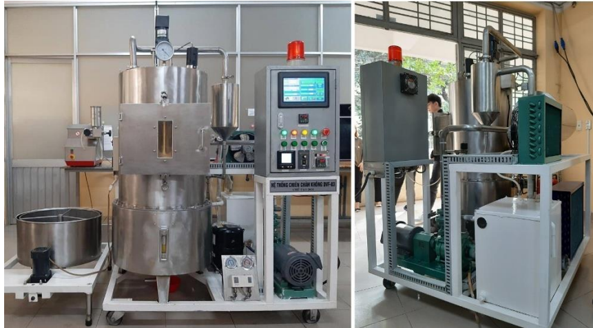
Figure 1. DVF-03 vacuum frying system with automated control, operated and monitored through a computer-based programmable system [10]
