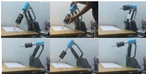
Figure 15. The robot is moved manually to separate points, and record them.
