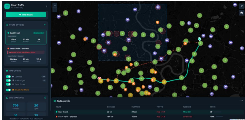
Figure 7. Web-based UI demonstration of the dynamic route optimization, illustrating the system actively avoiding a severely flooded segment.
