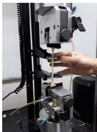
Fig. 2 Tensile Tester of INSTRON 5566 – CN 2081
