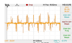
(b) Zero Common mode voltage PWM method with reduced current ripple [4]
