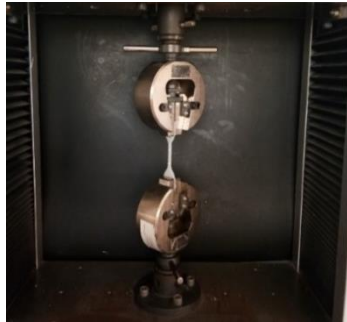
Fig.4. Placing sample for Tensile Strength Test
