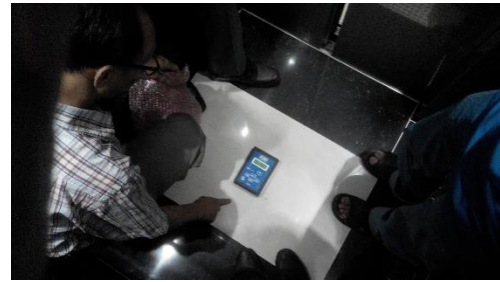
Figure 7. Elevator test tower in Long an (a), 3-axis accelerometer (b) and the accelerometer put on the elevator floor for measuring (c)
