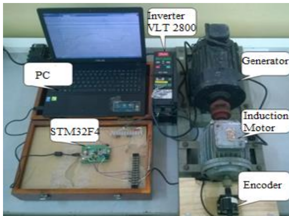
Figure 11. Image of practical motor speed control system
