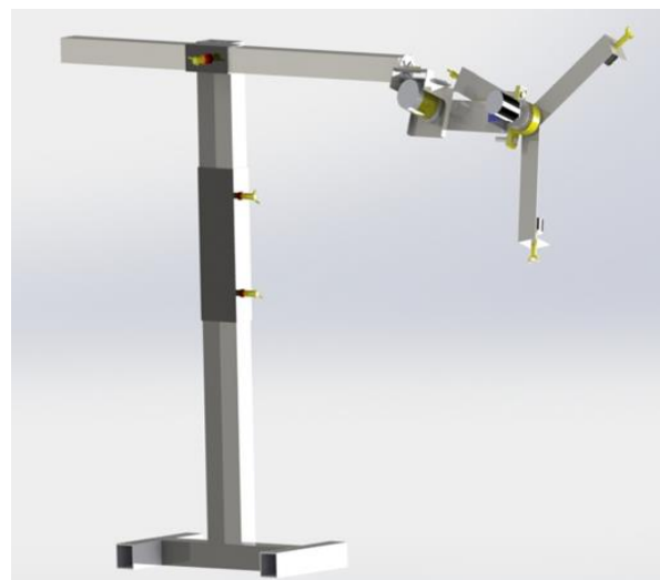
Figure 6. Driving mechanism & angle detecting
