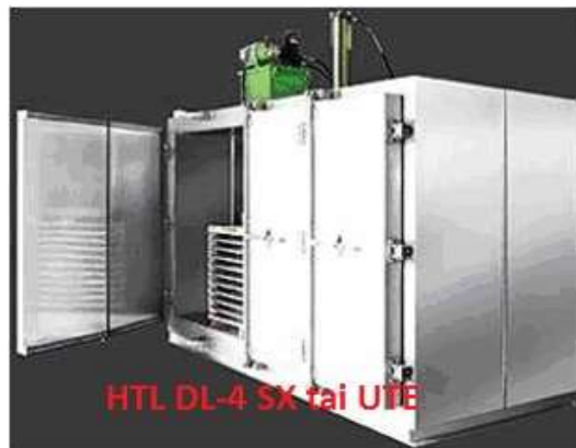
Figure 2. The Refrigeration system DL-4 with the auto freezing (-45 \div -40)^{\circ}C
