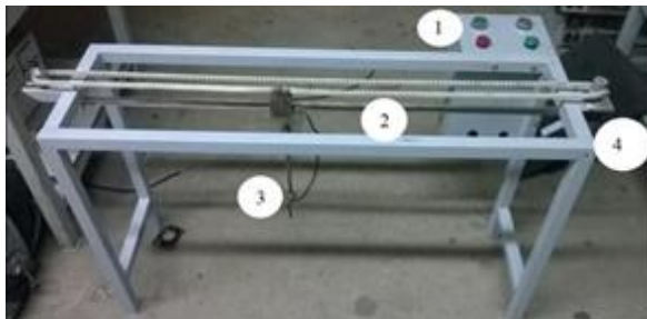
Fig. 7. Inverted pendulum on cart model in practice
