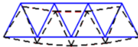
Fig. 13 The first-order natural mode of 15 bar truss: red color by FEM; black color by IGA.
