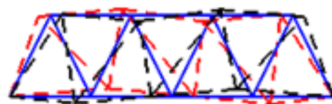
Fig. 15 The fourth-order natural mode of 15 bar truss: red color by FEM; black color by IGA.
