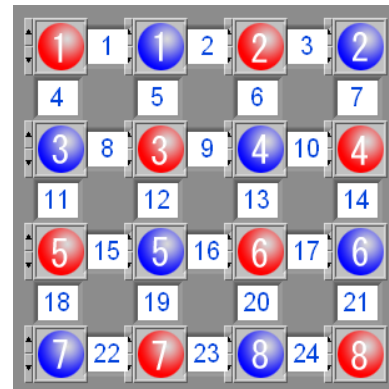
Figure 3. A matrix set up at the right brain side to obtain 24 fNIRS channels
