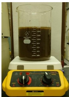
Figure 1. Activated sludge was washed with 1% (v/v) hydrochloric acid
