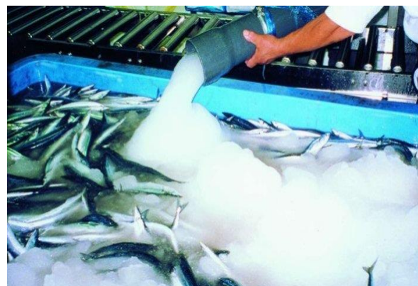
Figure 10. Slurry ice for fish preservation. [8]
