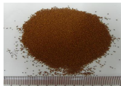
Figure 3. Iron-impregnated granular ceramics
