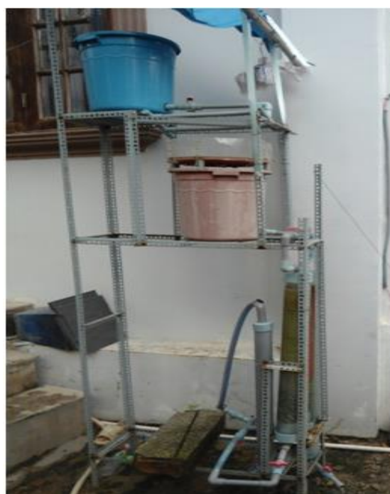
Figure 2. A household-scale drinking water treatment unit
