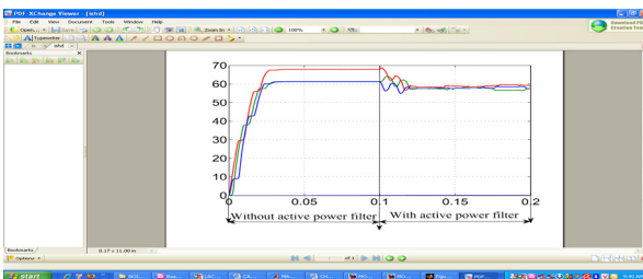
Fig.15. Diagrams of source effective three-phase current.
